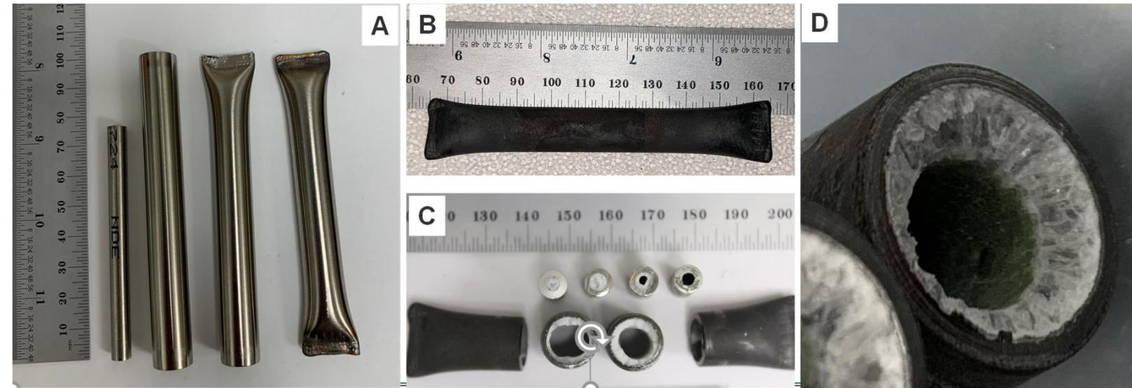
*SS316 test ampoules to determine chromium diffusivity.*
