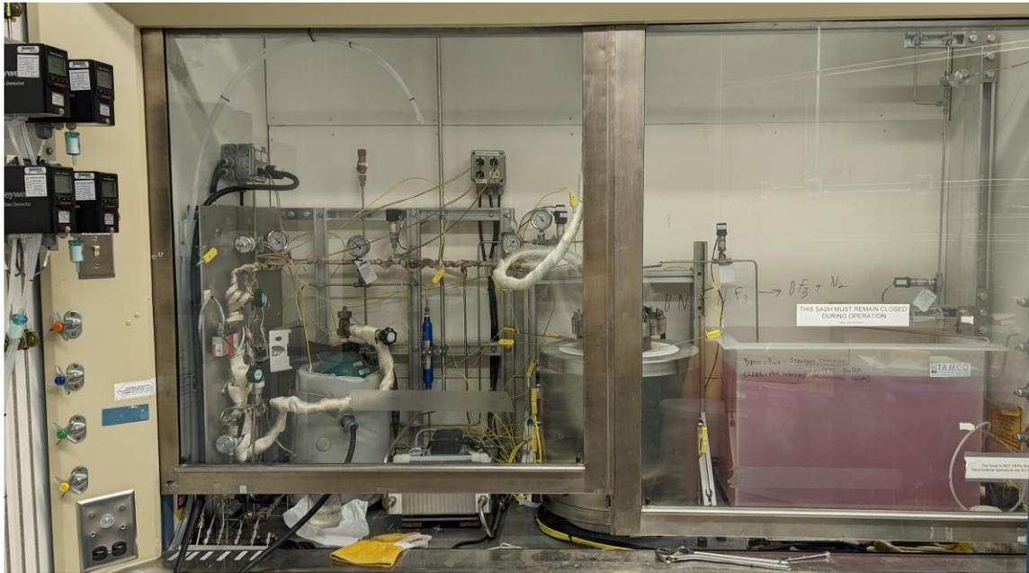
New fluoride salt purification system for exploring new purification processes (e.g. replacing HF with  $\text{NF}_3$ )
