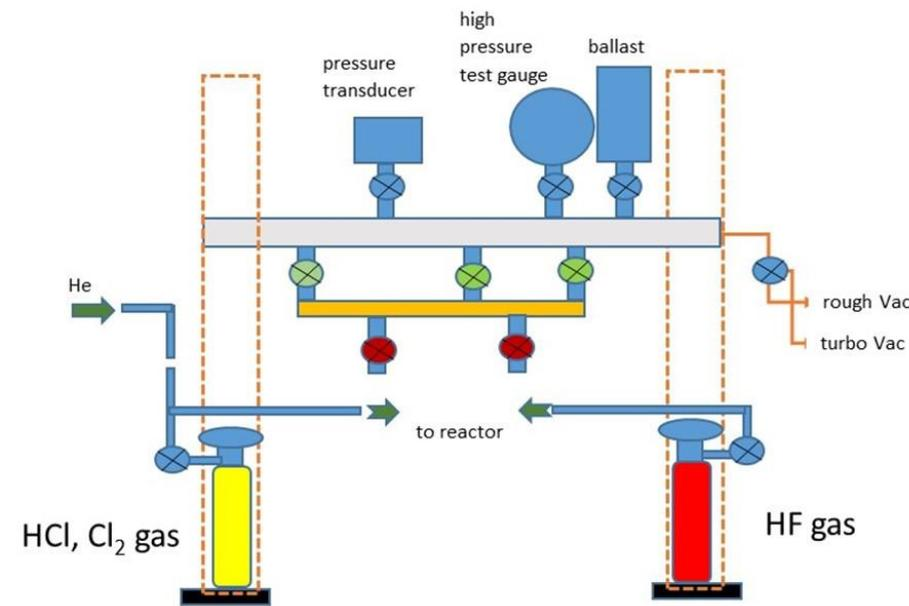
The vacuum line for preparation of fluoride and chloride salts
