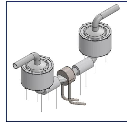
*8 Freeze Valves to accomplish fuel load/offload and reactor fill/drain*
