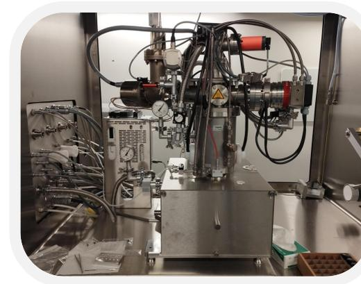
In-house radioactivity lab facilities (under commissioning), including gloveboxes with integrated furnaces (bottom) and thermal analysis instrument (top).
