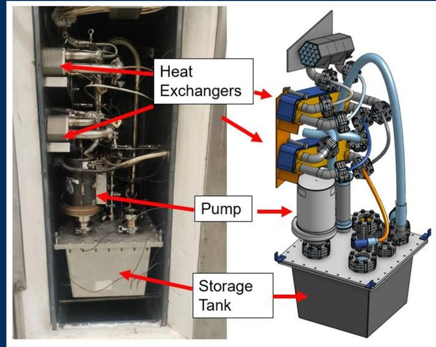
Picture (left) and drawing (right) of pumped loop
