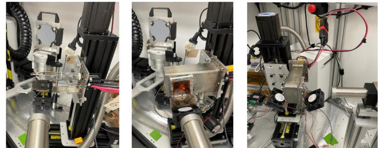
*Vacuum furnace for EasyXAFS 300 to allow for in-situ metal halide speciation under molten salt conditions.*
