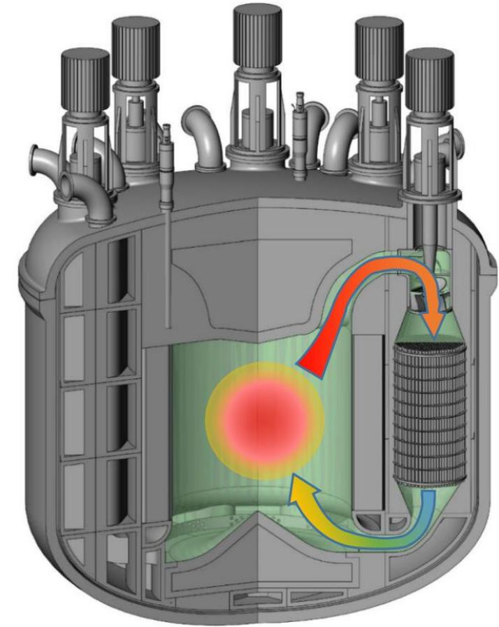
**Molten Chloride Fast Reactor [5]**
