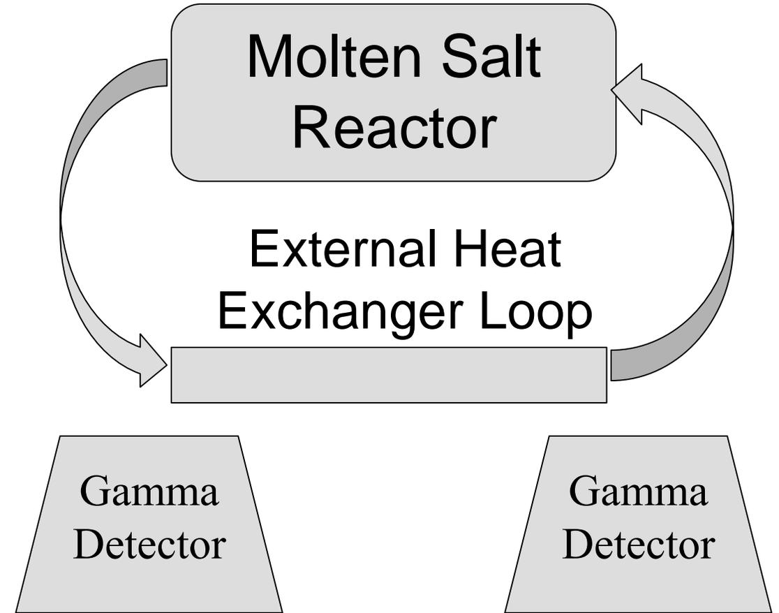
Can Measure Flow in Clean Salt with 11 Second F-20, 1633 KeV
