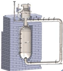
**Molten Chloride Reactor Experiment (MCRE)**
