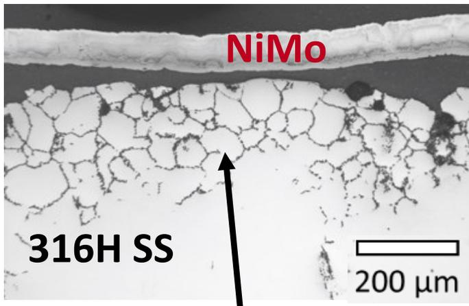
Substrate attack on 316H SS with functionally graded overlay
