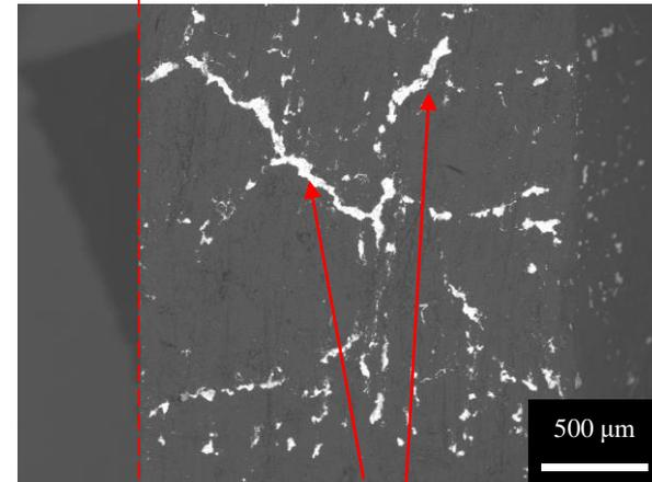
Salt-graphite interface      Salt-infiltration path
