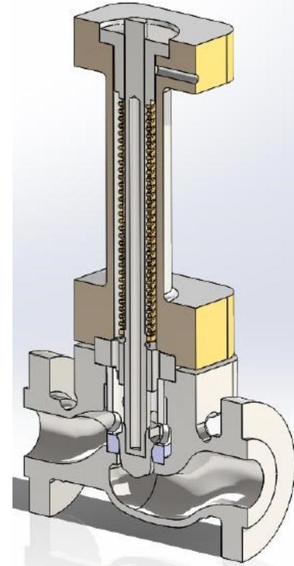
2" Flowserve valve for controlling flow of molten salts from Gen3 CSP
