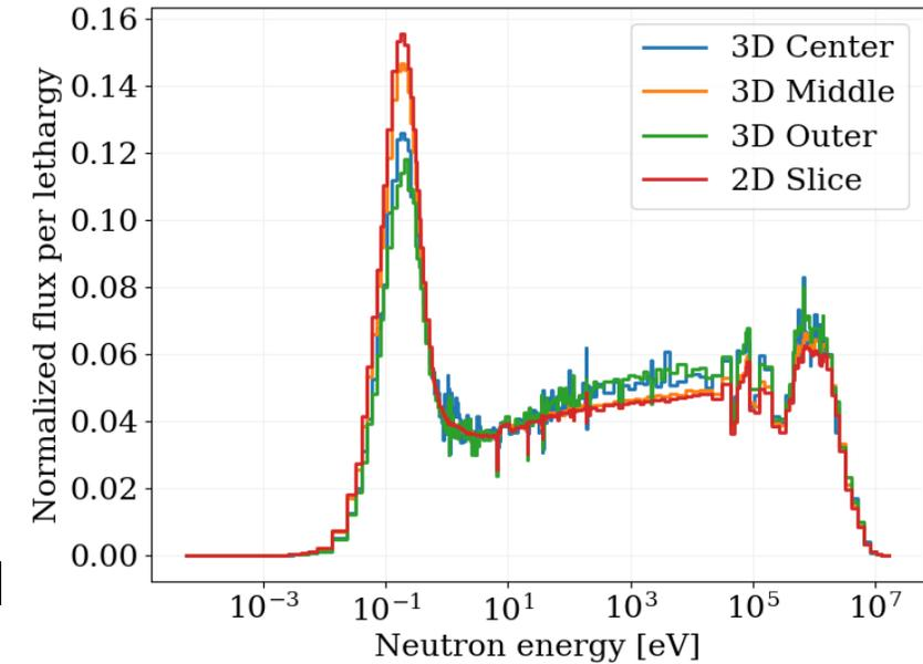
**Neutron flux comparison between 3D and 2D slice model**
