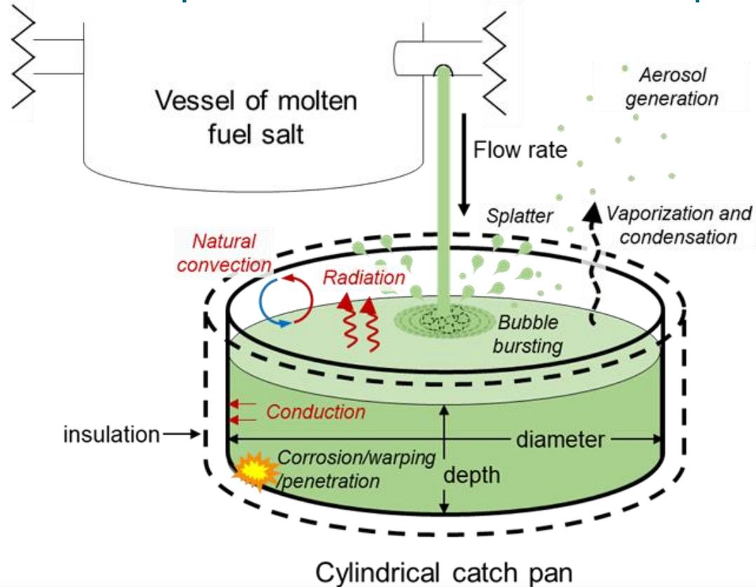
*Schematic of molten salt spill scenario being simulated in laboratory-scale tests*
