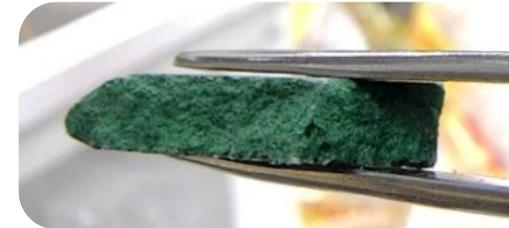
Solidified NaF-KF-UF<sub>4</sub> fuel (Fuel Qual. Experiment at INL)
