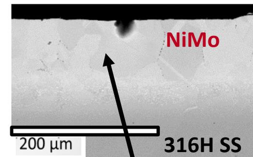
Functionally graded, diffusion bonded NiMo overlay
