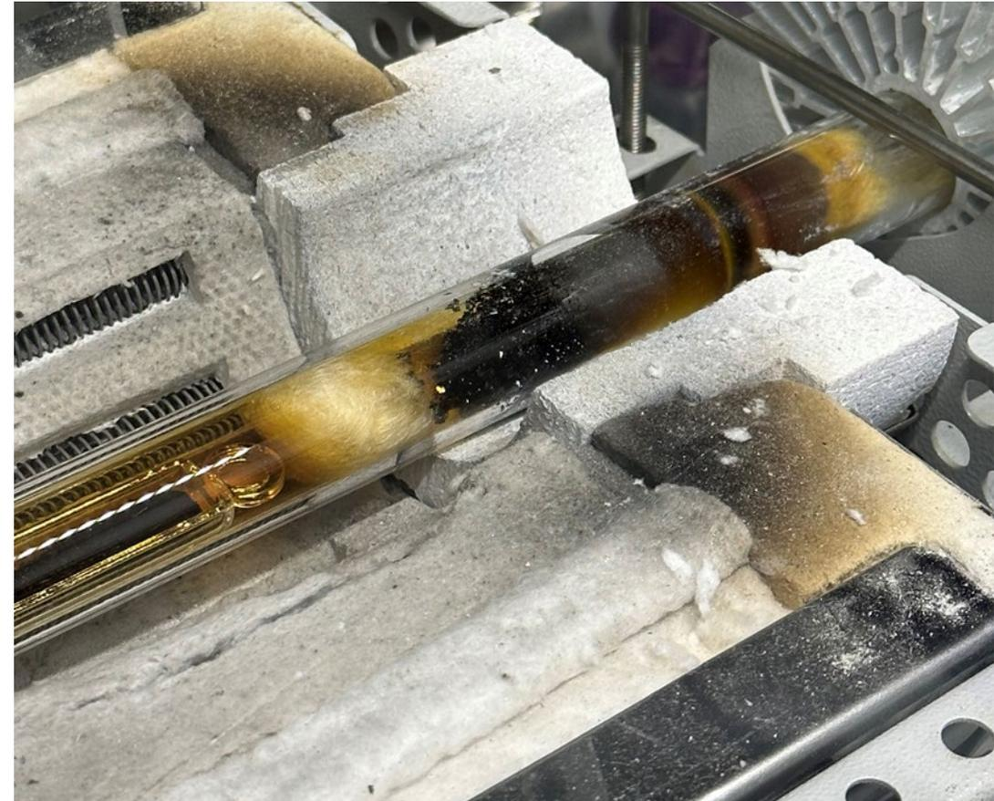
Uranium chloride in the gas phase (brown gas near the boat), solidified  $UCl_4$  (dark crystals just outside of the heated zone)
