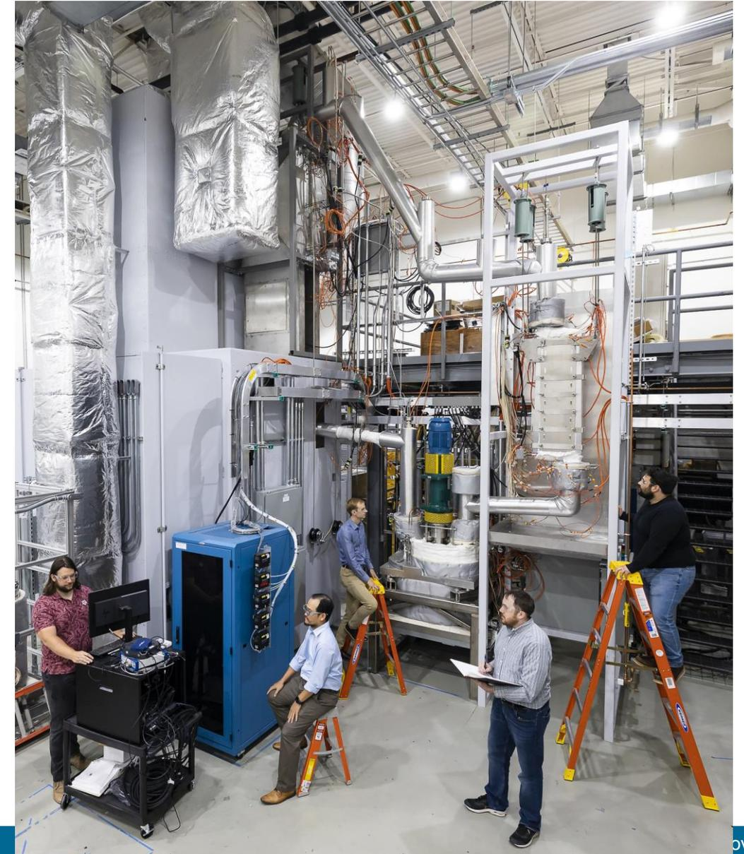
LSTL → pumped FLiNaK heated > 600°C
