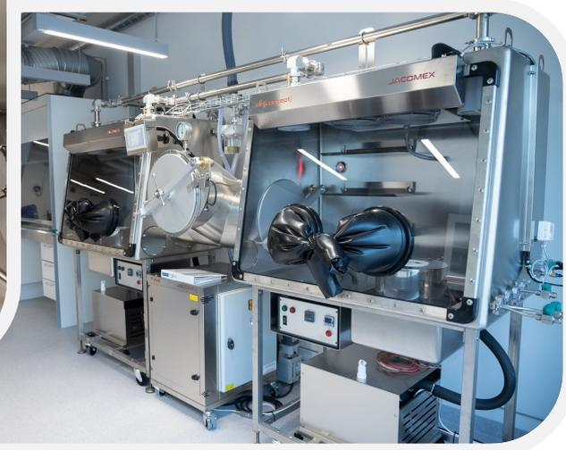
*In-house radioactivity lab facilities, including gloveboxes with integrated furnaces (right) and thermal analysis instrumentation (left).*
