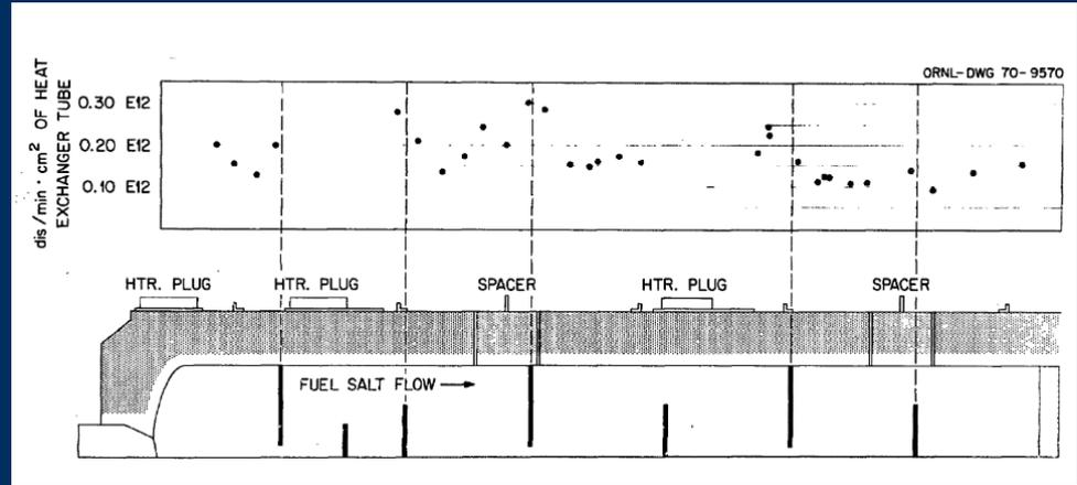
Activity of  $^{95}\text{Nb}$  at reactor shut down in the MSRE heat exchanger
