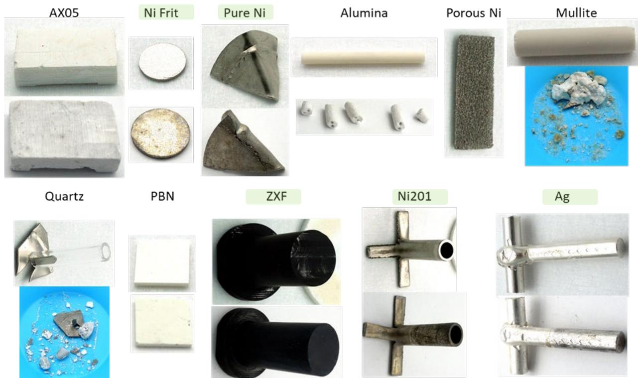
Sample images before/after 500-hours corrosion test at 750°C in FLiNaK
