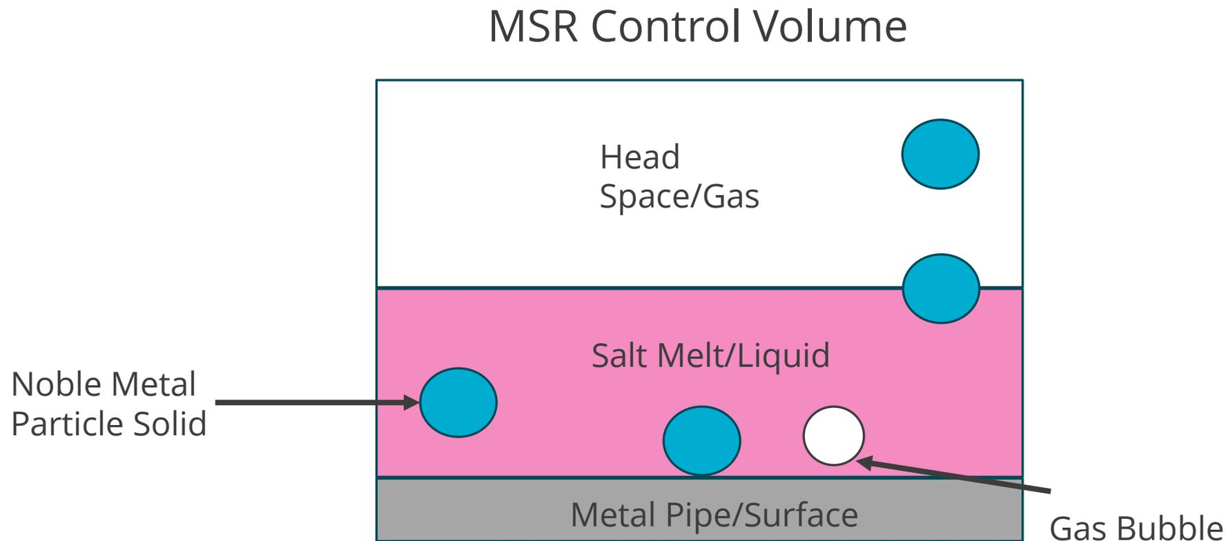
**Many different chemical processes can occur in one MELCOR control volume**
