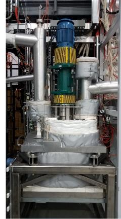
LSTL Pump >35 GPM, 20 ft alloy 600 FASTR Pump >70 GPM, 29 ft alloy C-276
