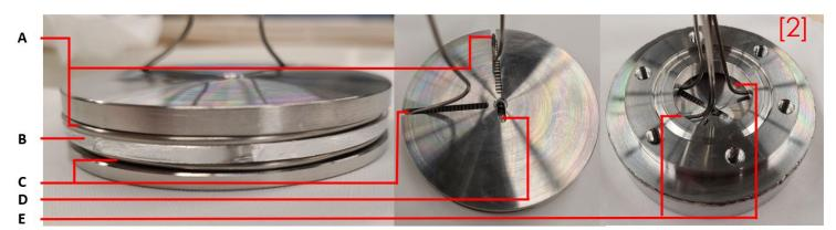
(A) axial guard heater, (B) quartz insulator, (C) main heater,(D) center thermocouple slot, and (E) side thermocouples placed in welded heater assembly cup
