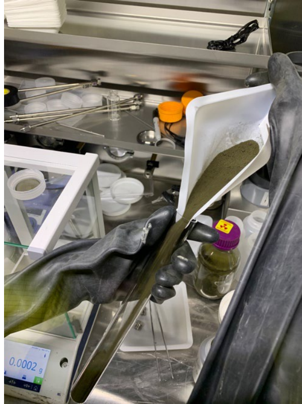
UCl 3 -salt mixture loading for viscosity experiment
