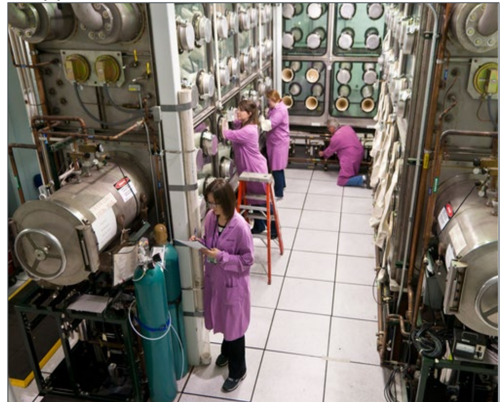
Thermophysics laboratory with equipment located in Ar-atmosphere radiological gloveboxes
