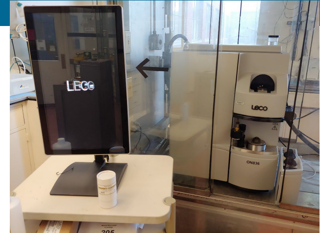
LECO measurement of oxide concentration in molten salt including beryllium salts
