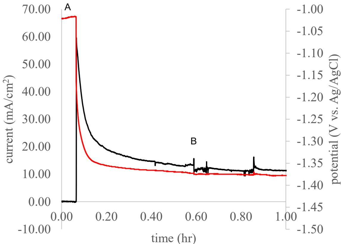
**A:** Insertion of Zr rod (WE), **B:** attempted addition of  $\text{NiCl}_2$
