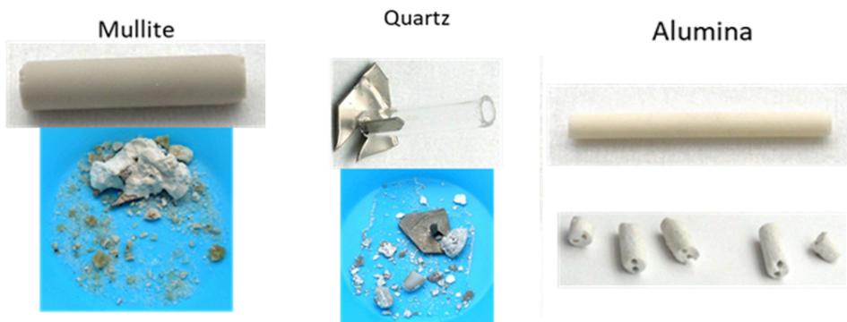
Sample images before/after 500-hours corrosion test at 750°C in FLiNaK
