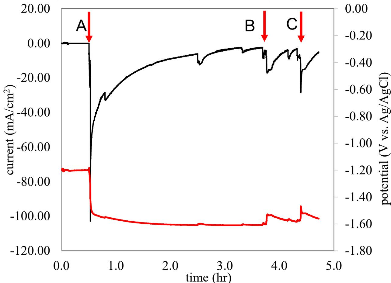
**A:** Insertion of Zr rod (CE), **B:** 1<sup>st</sup> addition of  $\text{NiCl}_2$ , **C:** 2<sup>nd</sup> addition of  $\text{NiCl}_2$
