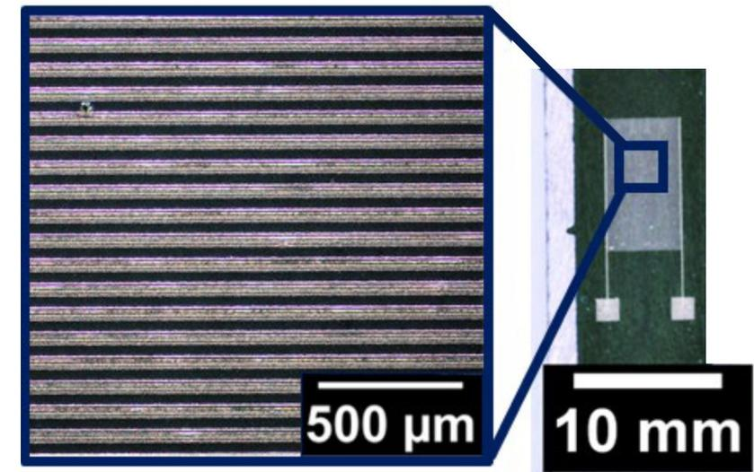
Strain gauge printed at BSU
