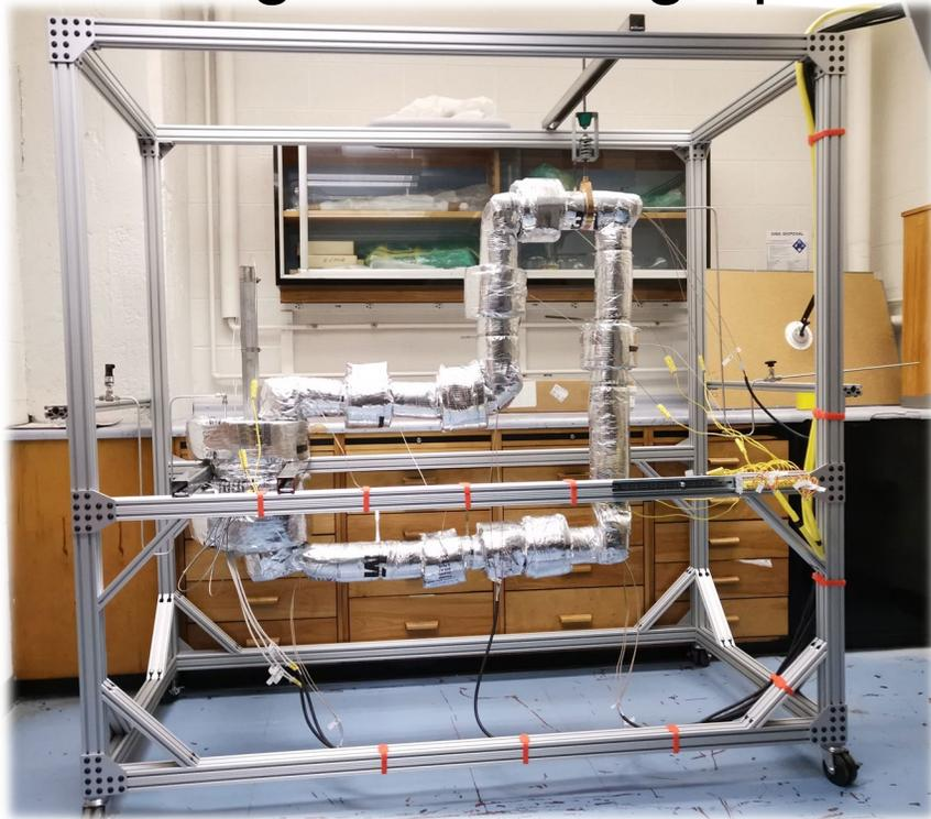
Neutron irradiation loop with Flibe salt and experiments in the M<sup>3</sup> Facility
