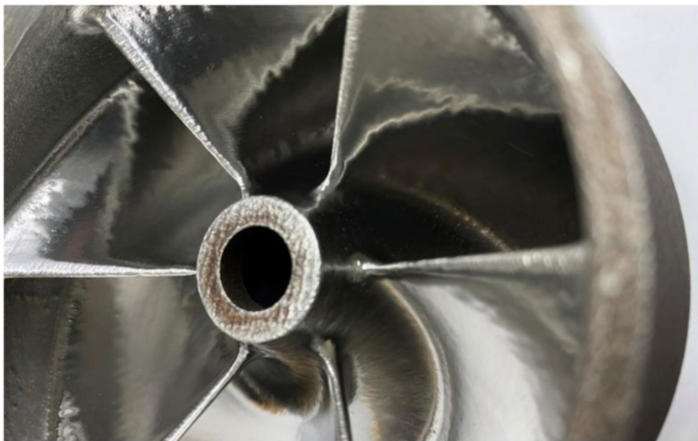
At the Department of Energy Manufacturing Demonstration Facility at ORNL, this part for a scaled-down prototype of a reactor was produced for industry partner Kairos Power. Credit: Kairos Power
