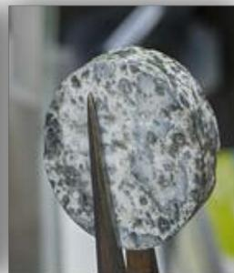
FLiBe with TCP (partially reacted)
