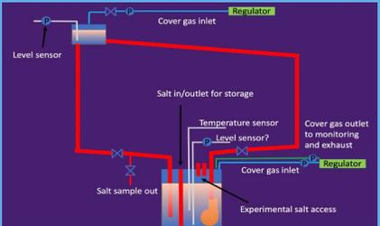
Fluoride Molten Salt Test Loop
