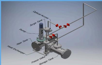
Molten Salt Test System
