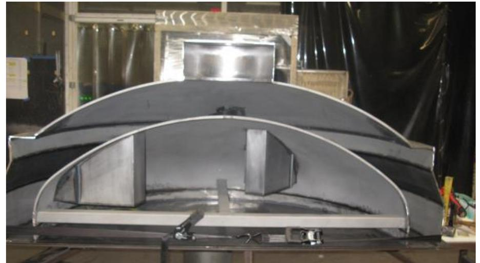
Note: Two reactor internals support structures
