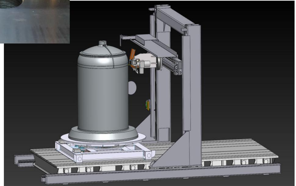
Lower Flange Shell Mockup EB Weld -- ~6 ft (1.82m) diameter (Note, mockup is upside down)
