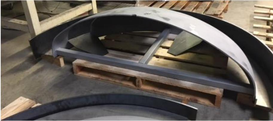
3/8-inch (9.5mm) thick lower head construction;
