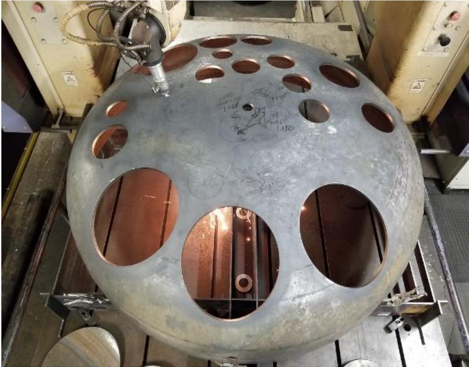
Laser machining of the penetrations to attach CRD nozzles
