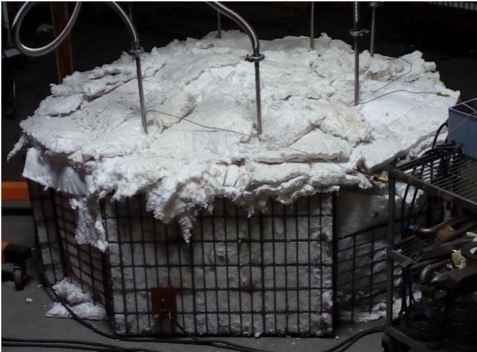
Hot Degassing of Powder Filled Upper Head
