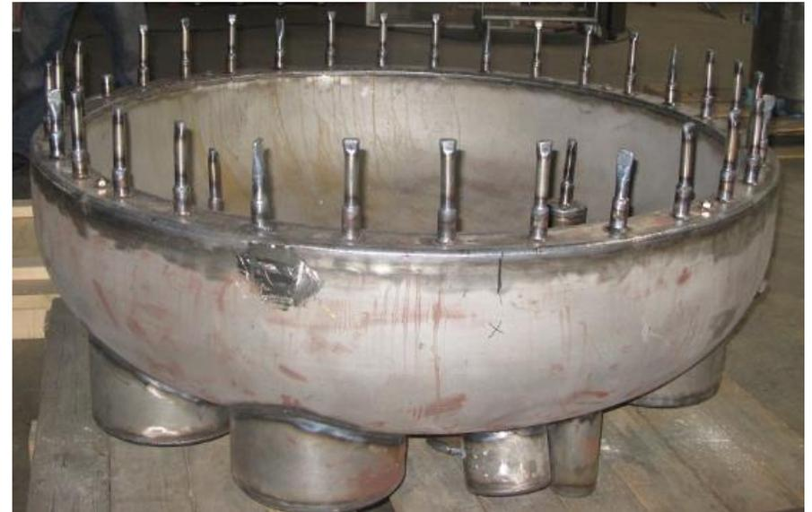
Following Degassing, All Fill Stems are Crimped and Welded Shut. Now Ready for HIP
