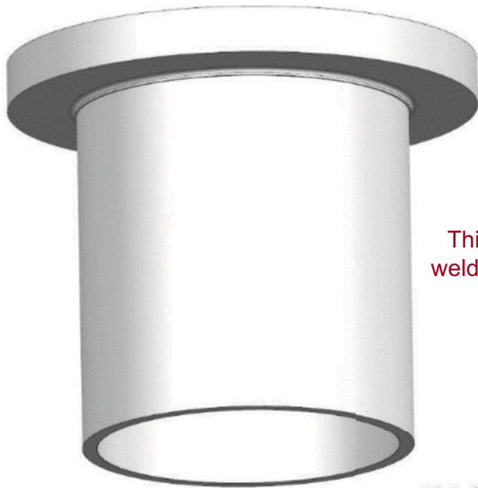
Thick flange to be welded to lower shell via EBW
