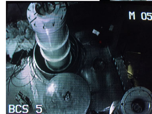
Lowering a loaded Liner down thru Bottom Loading Port and into TN-RAM cask
