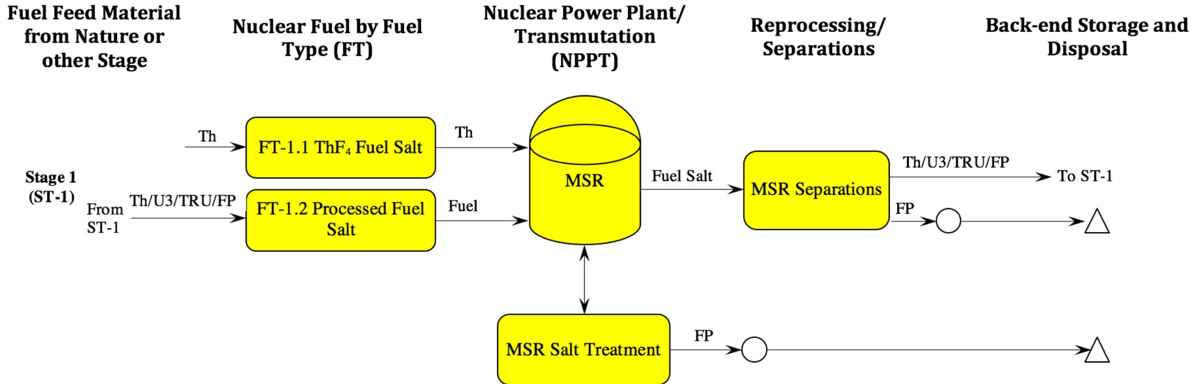
Continuous recycle of  $^{233}\text{U}/\text{Th}$  with new Th fuel in thermal critical reactors
