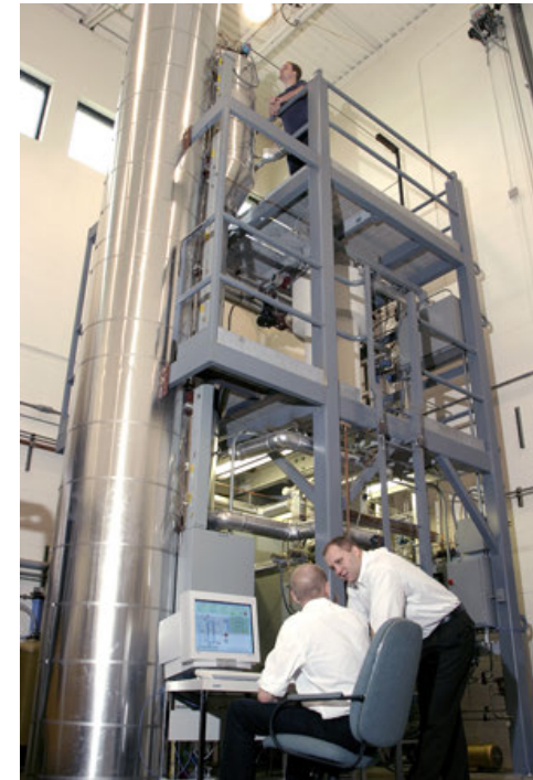
MASLWR IET facility, Oregon State University, Reduced height (1/3), reduced area (1/255 volume), 0.60 MW (NuScale)
