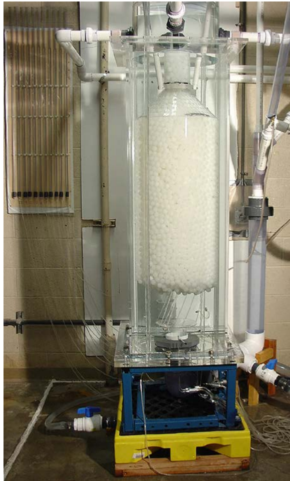
2006: UCB Pebble Recirculation Experiment (PREX)
