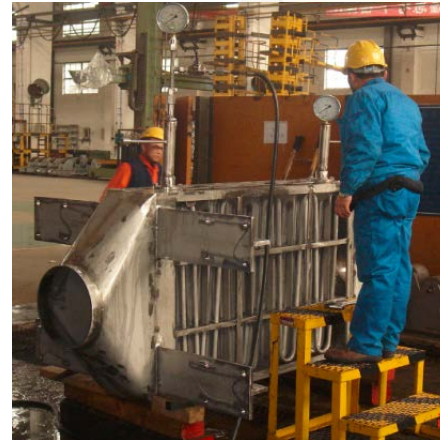
Principle prototype of molten salt pump and salt-air heat exchanger
