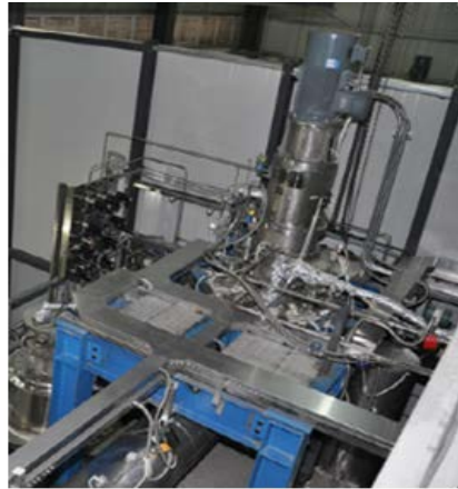
Principle prototype of molten salt pump and salt-air heat exchanger
