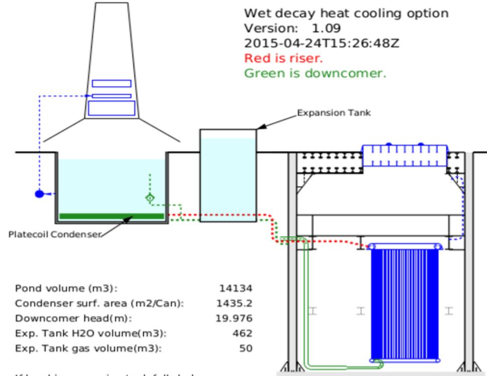
If level in expansion tank falls below level in pond, pond check valve automatically drains portion of pond water into membrane wall loop.
