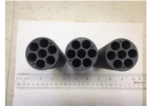
Six Compartment Graphite Crucible for Corrosion Tests
