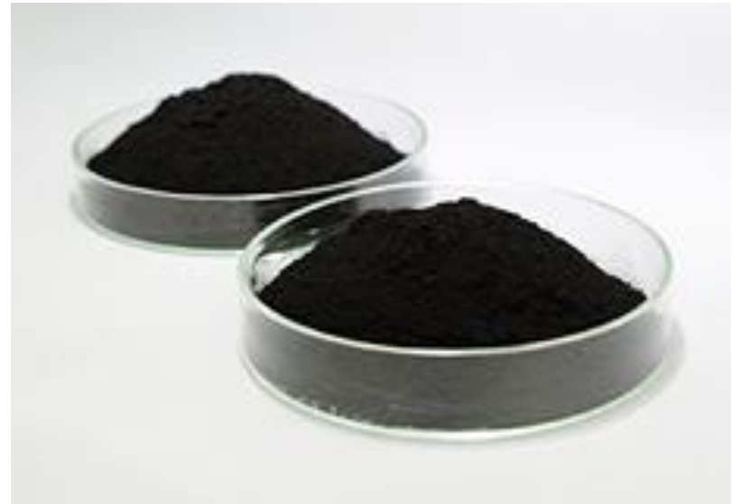
Platinum on High-Surface-Area Carbon (Commercial Catalyst for Hydrogenation Reactions)
