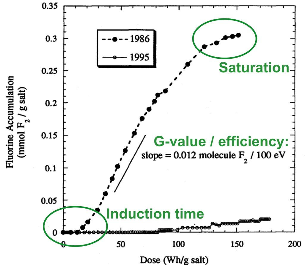
Fig. 3. Fluorine generation curves for 1986 and 1995 irradiation experiments.
