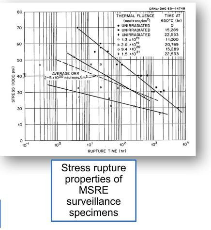
All niobium-modified Alloy N specimens irradiated at 650°C had rupture lives in excess of those of standard unirradiated Alloy N
