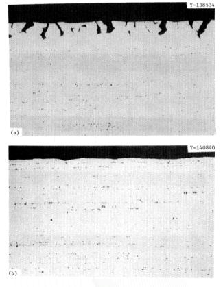
Alloy N exposed to MSRE fuel salt (500 h, 700°C) containing tellurium (a) oxidizing, (b) reducing – 100x
