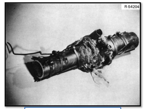
Bottom of cracked freeze valve
