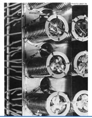
Cluster of modified Alloy N creep specimens prior to irradiation
